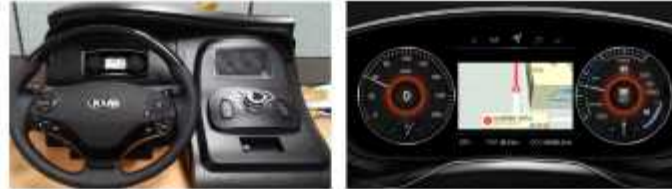
Fig. 18. Automotive digital cluster hardware and display.
